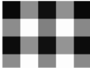
Figure 20: Raw data of image; Black are blue pixels, Gray are Green Pixels, White are Red
